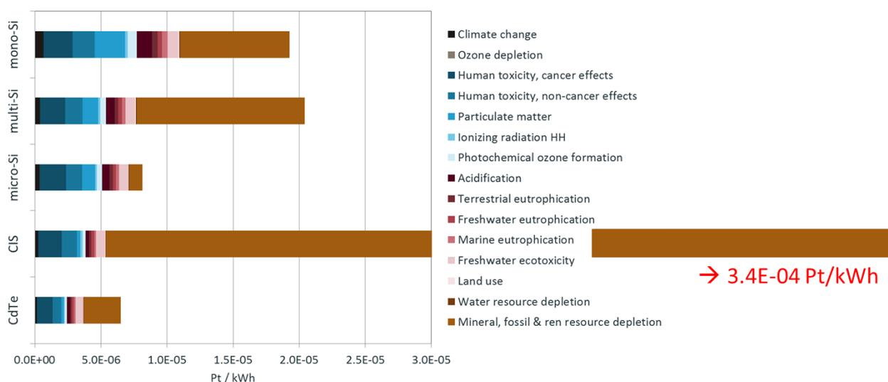
Figure 1 Cumulative weighted results of 3 kWp PV systems mounted on a slanted roof based on the PEF screening study (Stolz et al. 2016) as presented at the 2<sup>nd</sup> SC meeting in Brussels on 30.09.2015.
